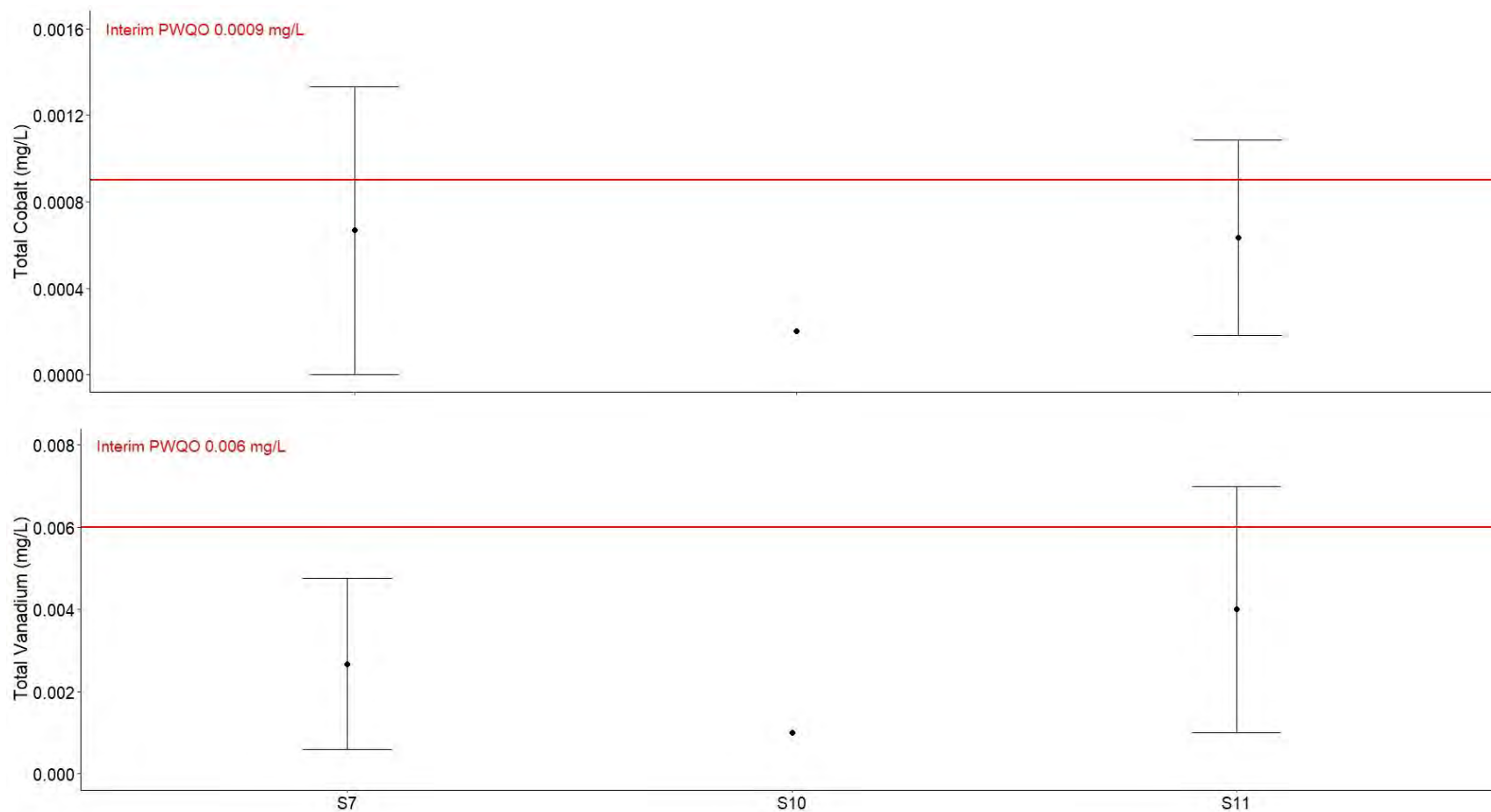
Figure B7 Total Cobalt and Total Vanadium concentrations in the water samples collected from Ramsay Creek. The red line dictates the Provincial Water Quality Objectives (PWQO) values. The whiskers depict the standard deviation
