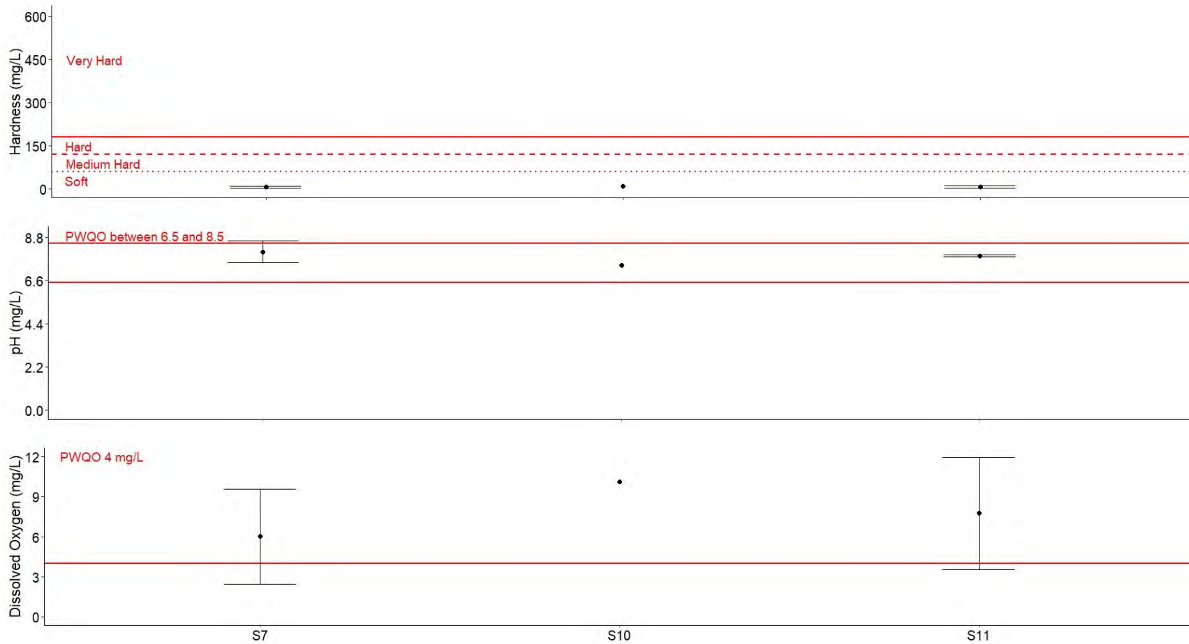
Figure B5 Harness, pH, and Dissolved Oxygen concentrations in the water samples collected from from Ramsay Creek. The red line dictates the Provincial Water Quality Objectives (PWQO) values. The whiskers depict the standard deviation
