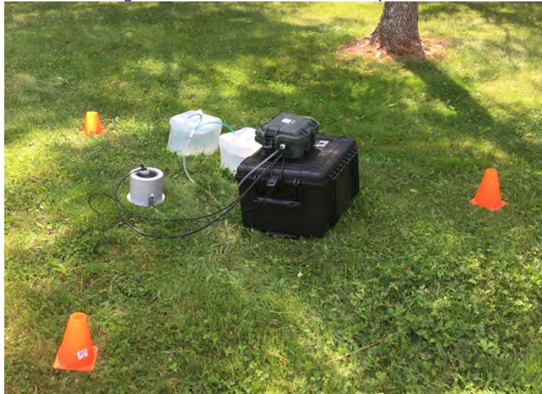
Figure 7: Infiltration Test Setup, 2022
