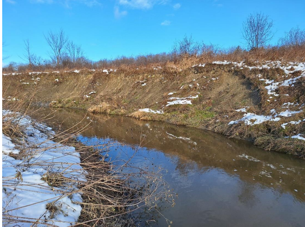
Large cutfaces were observed where the channel came in contact with the edge of agricultural fields. Basal scour was observed along both banks throughout the reach.
